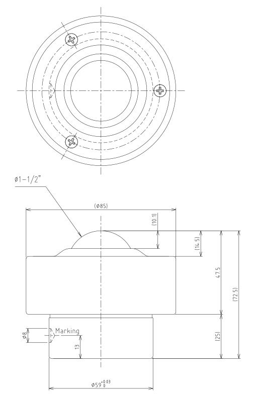
>Description S Type Stroke Ball Transfer S-38 Type Unit = mm
