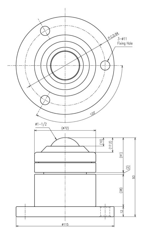
>Description IS-BF Type Spring Ball Transfer IS-38BF Type Unit = mm
