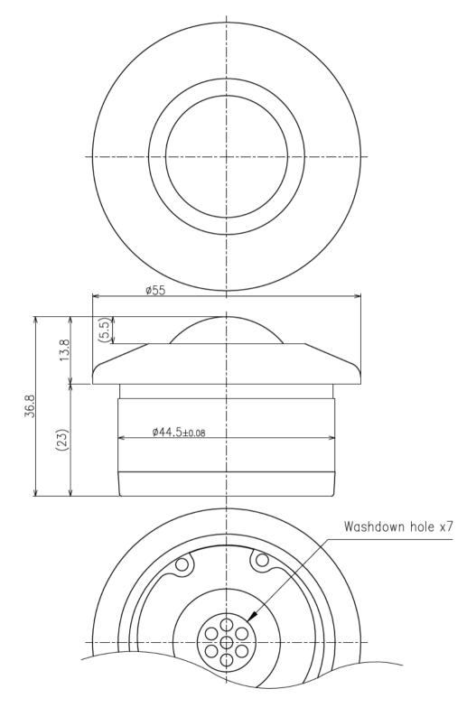
>Description IS-D Type Ball Transfer IS-30D Type Unit = mm
