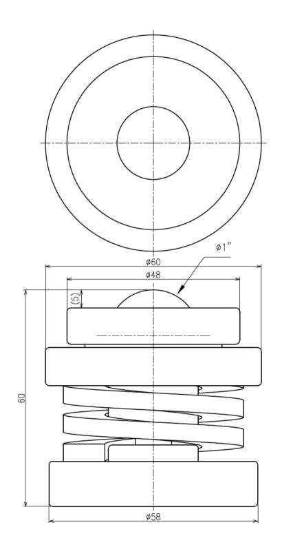
>Description IS-BK Type Spring Ball Transfer IS-25BK-20 Type Unit = mm
