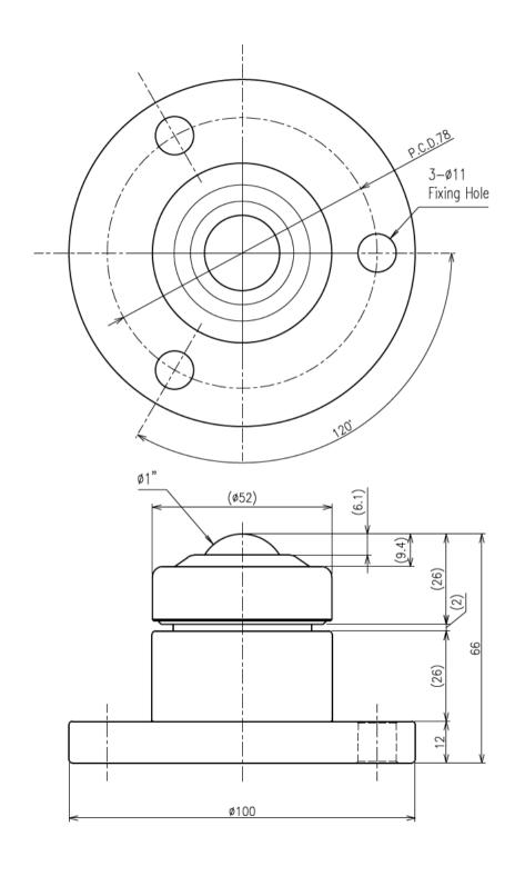
>Description IS-BF Type Spring Ball Transfer IS-25BF Type Unit = mm
