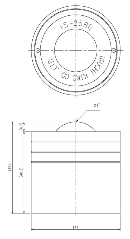
>Description IS-BD Type Spring Ball Transfer IS-25BD Type Unit = mm
