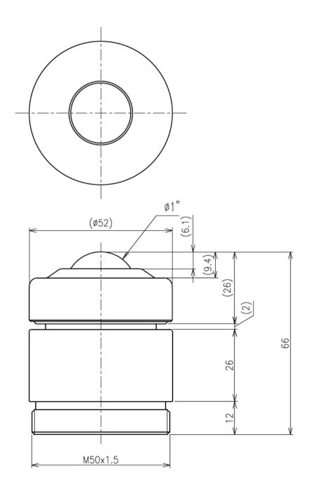
>Description IS-B Type Spring Ball Transfer IS-25B Type Unit = mm
