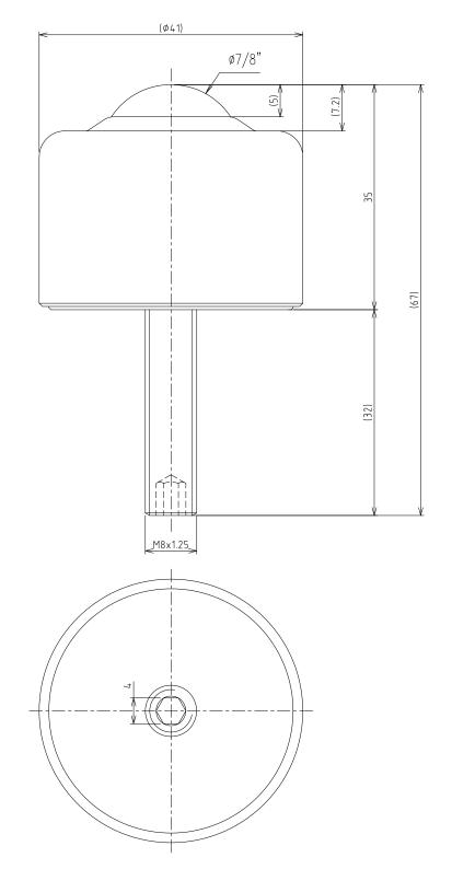
>Description IS-SN Type Ball Transfer With Sturdy Bolt IS-19SN Type Unit = mm
