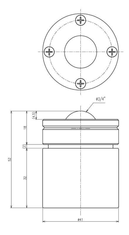
>Description IS-BM Type Spring Ball Transfer IS-19BM Type Unit = mm
