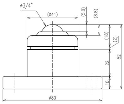
>Description IS—BF Type Spring Ball Transfer IS—19BF Type Unit = mm
