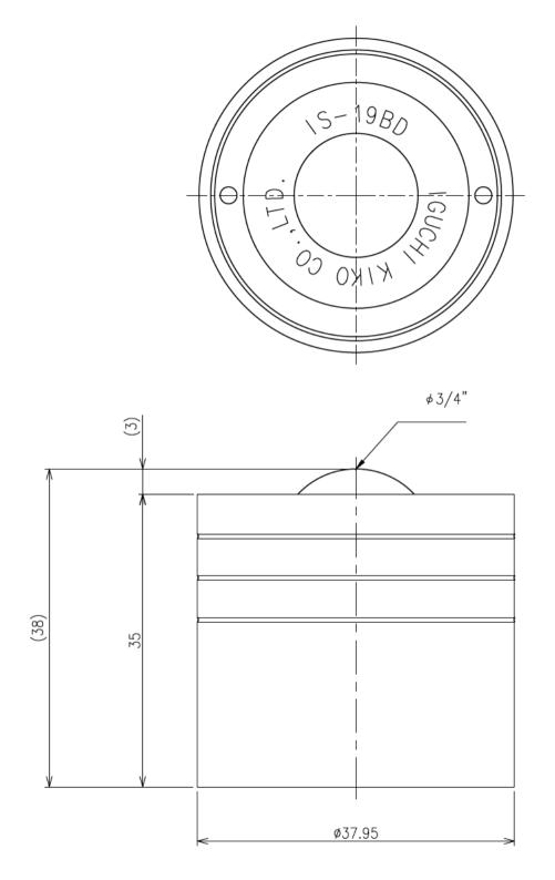
>Description IS-BD Type Spring Ball Transfer IS-19BD Type Unit = mm
