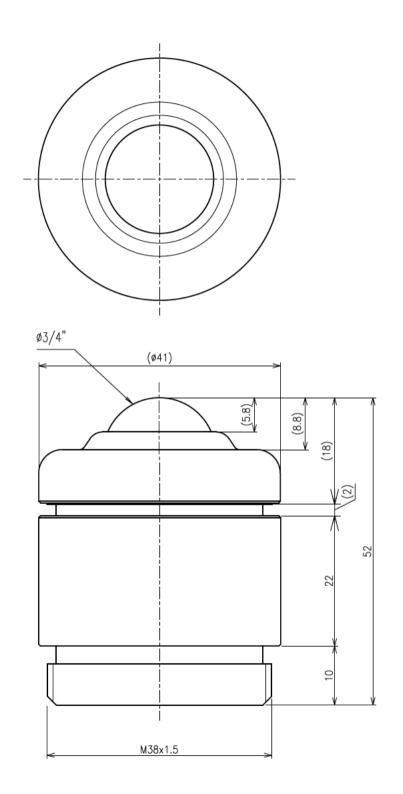
>Description IS-B Type Spring Ball Transfer IS-19B Type Unit = mm
