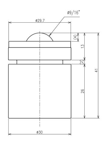
>Description IS—BM Type Spring Ball Transfer IS—14BM Type Unit = mm
