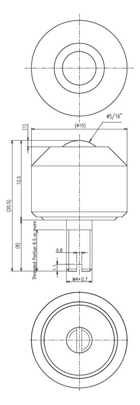
>Description IS—SNM Type Ball Transfer With Sturdy Bolt IS—08SNM Type Unit = mm
