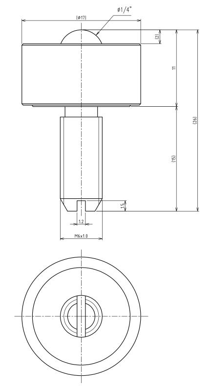
>Description IS-SN Type Ball Transfer With Sturdy Bolt IS-06SN Type Unit = mm
