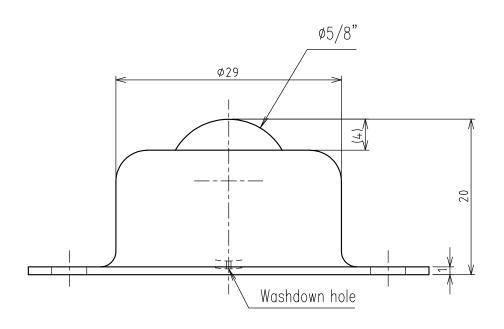
>Description IM-J Type Ball Transfer IM-16J Type Unit = mm
