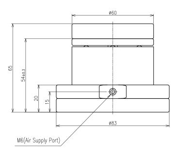
>Description ILS—S Type Positioning Stage ILS—30S—60 Type Unit = mm
