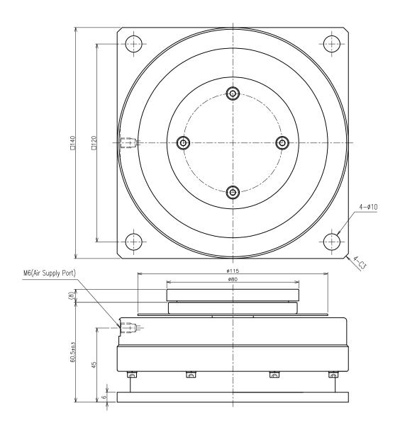
>Description ILS—S Type Positioning Stage ILS—150S—S20 Type Unit = mm
