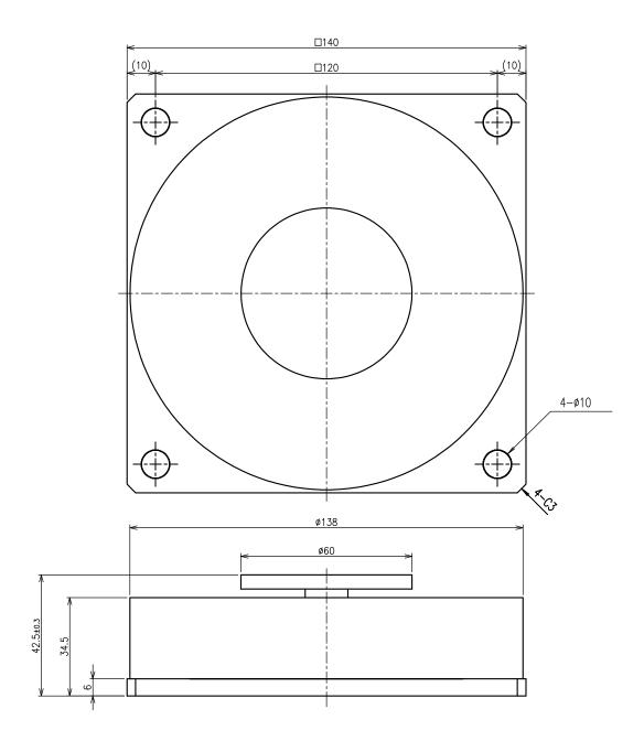
>Description ILS Type Positioning Stage ILS-150 Type Unit = mm
