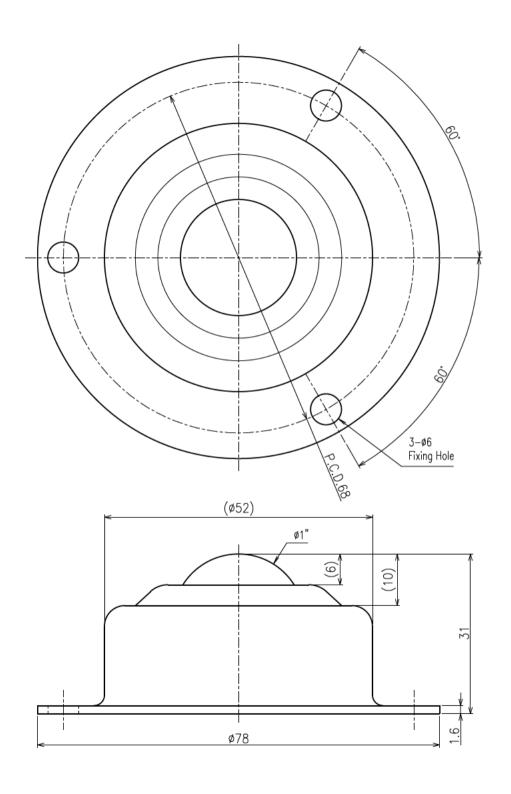
>Description IB—S Type Ball Transfer IB—25S Type Unit = mm
