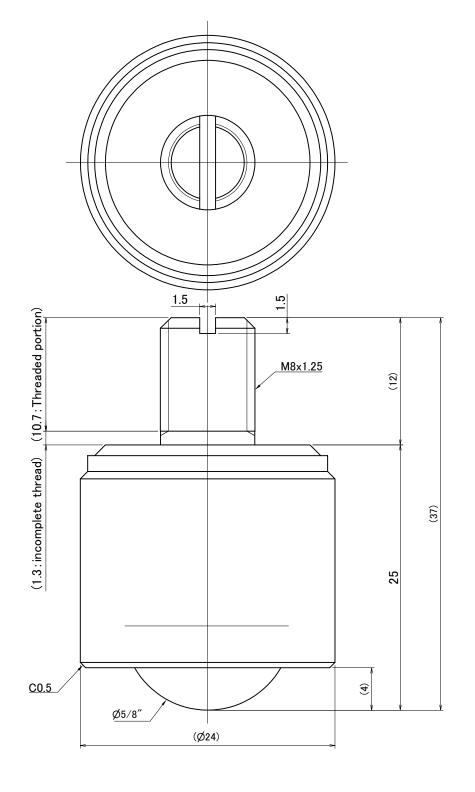
>Description CP-D Type Ball Transfer With Sturdy Bolt CP-16D Type Unit = mm
