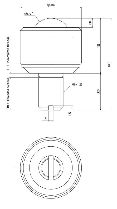
>Description CP-H Type Ball Transfer With Sturdy Bolt CP-13H Type Unit = mm
