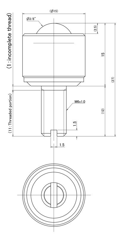
>Description CP-H Type Ball Transfer With Sturdy Bolt CP-09H Type Unit = mm
