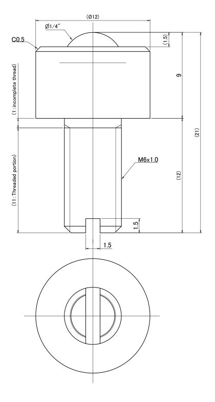
>Description CP-H Type Ball Transfer With Sturdy Bolt CP-06H Type Unit = mm
