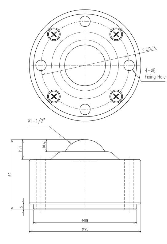
>Description IS-S Type Ball Transfer IS-38S Type Unit = mm
