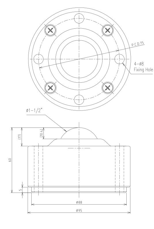
>Description IS Type Ball Transfer IS-38 Type Unit = mm
