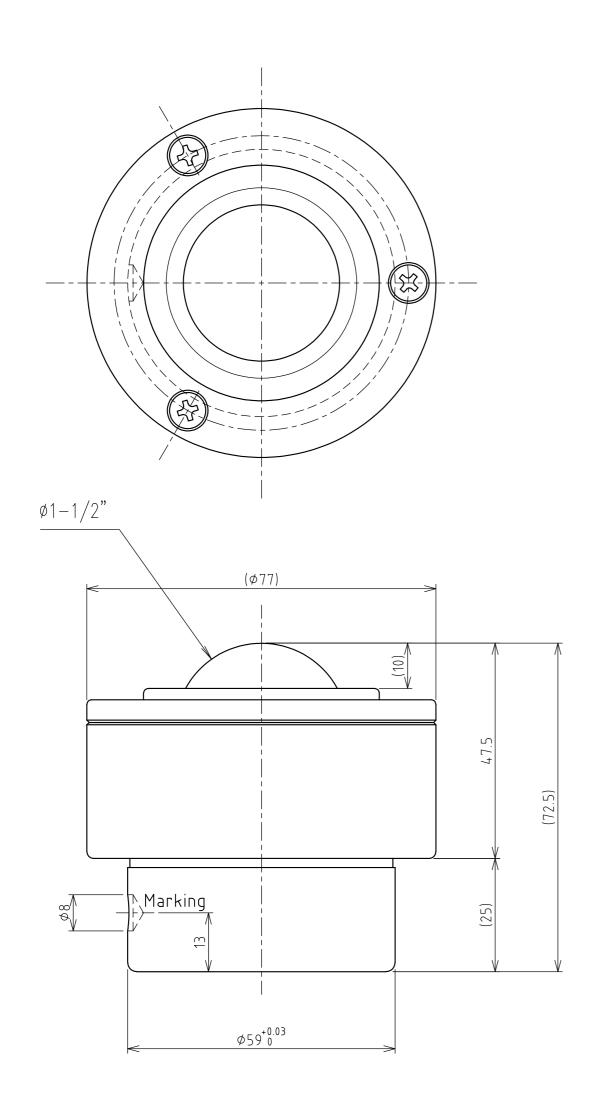
>Description S Type Stroke Ball Transfer S-38 Type Unit = mm
